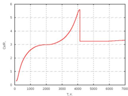
The heat capacity of nitrogen ( $N_2$ ), the internal energy and heat capacity of condensed carbon (graphite, liquid carbon).
