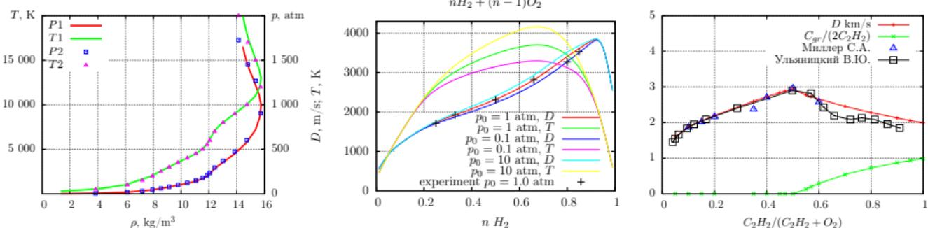
Shock wave in the atmosphere. Detonation of mixtures of hydrogen and acetylene with oxygen ( $D = u + c$ ).
