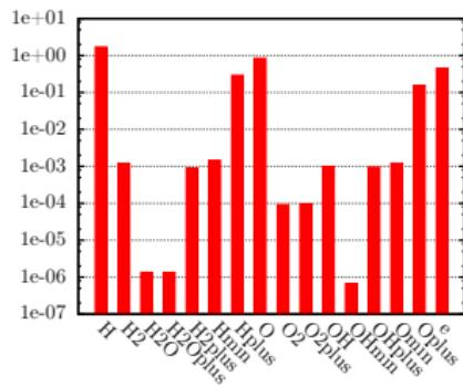
Equilibrium chemical concentrations of a mixture of gases with a composition of  $2H + O$  (water) at a temperature of 300, 3000 and 20 000 K. The density is 1 kg/m<sup>3</sup>.
