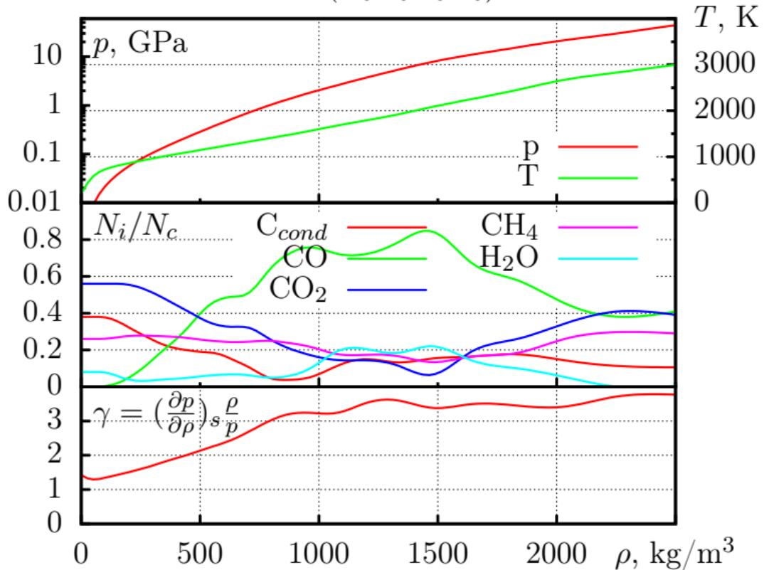
Adiabat unloading of detonation products (benzo three furoxane,  $\rho_0 = 1860$  kg/m<sup>3</sup>)
