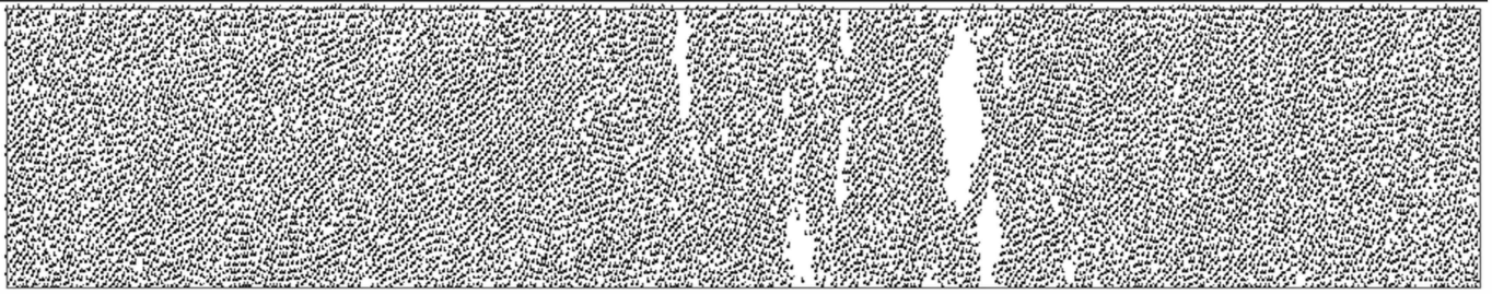
Fig. 1. Spinodal decay of a polar dielectric liquid in a high electric field. The MD ensemble consists of 11000 particles.
