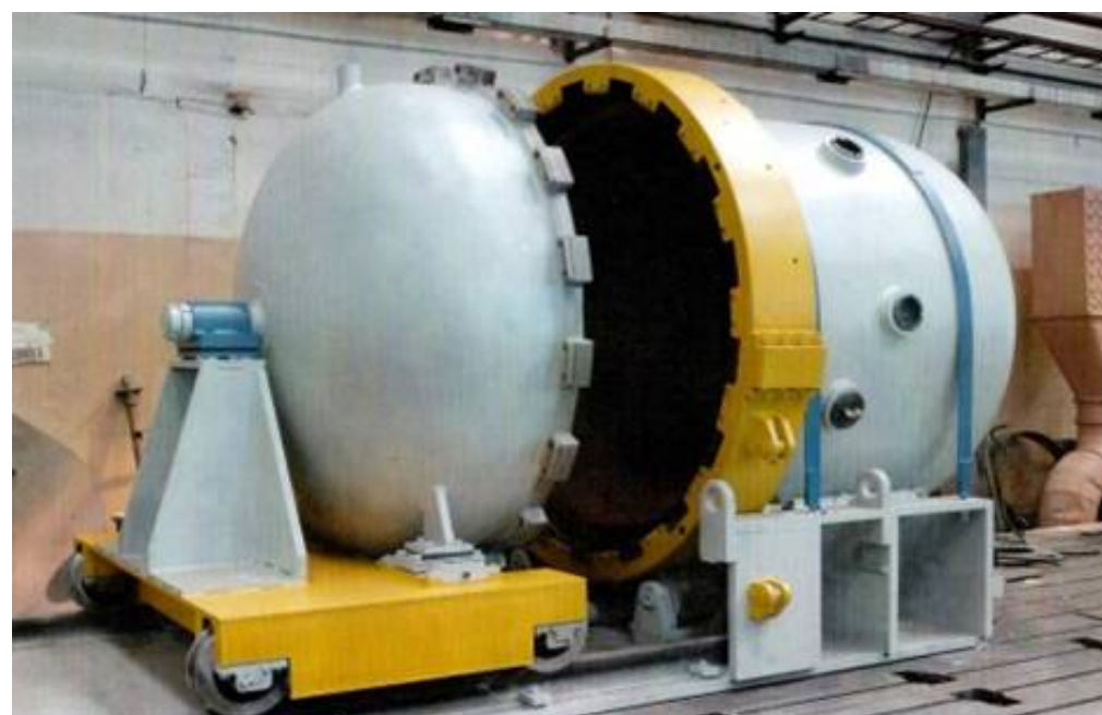
Explosion chamber for 2 kg of HEMs
